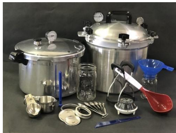
Figure 18. Pressure canner. Never process low acid vegetables or meat in a boiling water canner. A pressure canner must be used.
